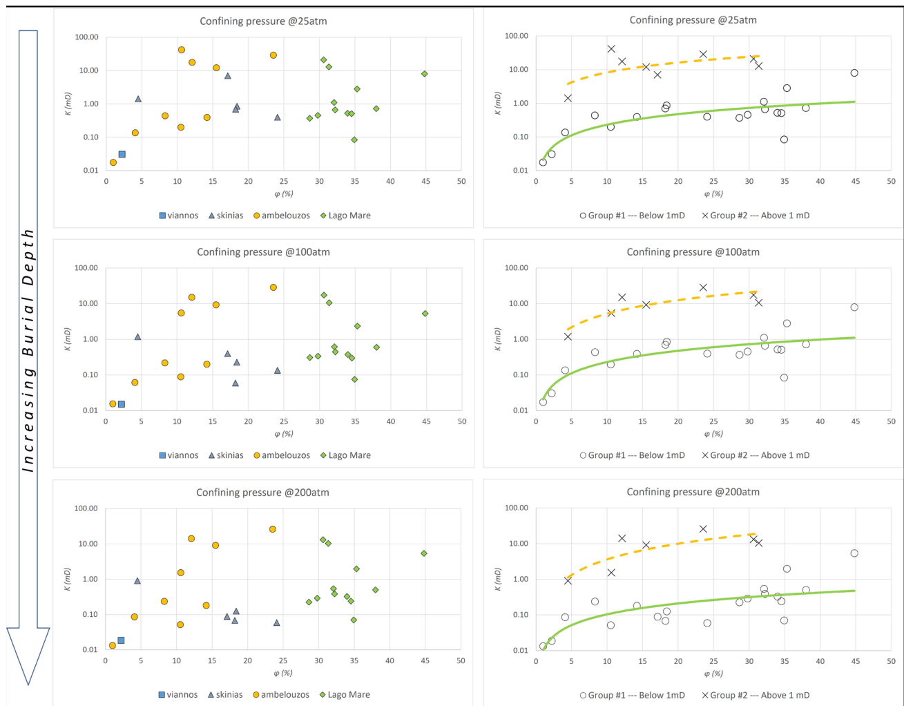
Fig. 9 Poro/permeability diagrams of outcrop samples in Messara basin (for location see Fig. 1). From top to bottom, the graphs illustrate the porosity and permeability values measured under the three different confining pressures of 25, 100, and 200 Atm, respectively. In the left column, the
